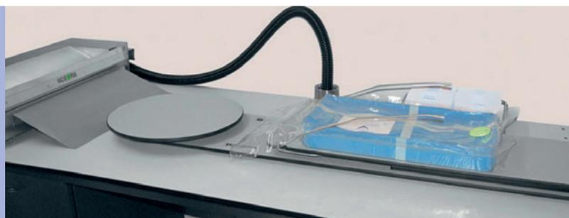
Using the turntable, the open end of the pouch is slid over two metal rods which open the pouch up as it is pulled forward so that it easily covers the wrapped set. The
