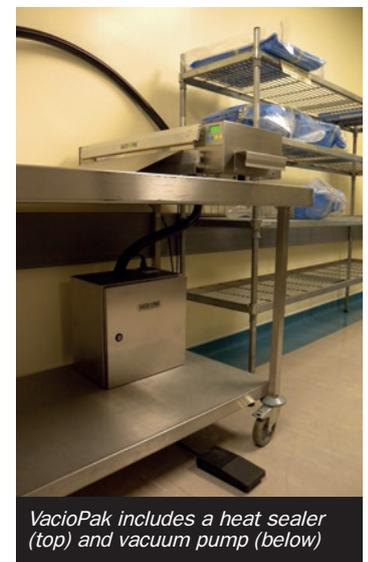
*VacioPak includes a heat sealer (top) and vacuum pump (below)*
